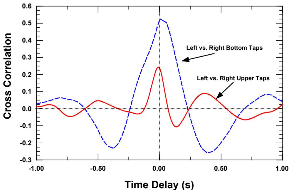
**Figure 4.** Cross correlation between taps on opposite sides of the bed when the bubble plume is shifted to the left. The fluidizing condition is the same as in **Fig. 3**.
