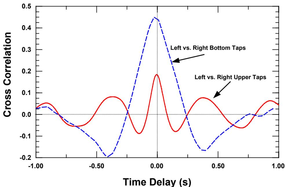
**Figure 3.** Cross correlation between taps on opposite sides of the bed when the bubbles are uniformly distributed. The fluidizing air flow was 2.35 times minimum.
