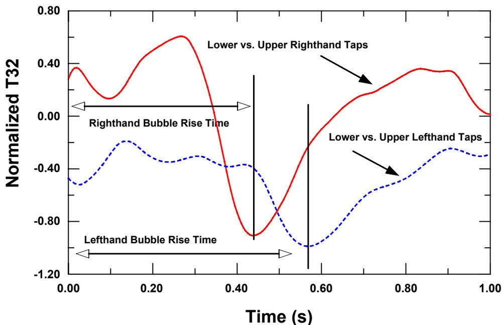
**Figure 6.** Time asymmetry between vertically spaced pressure taps. Bubble plume is shifted to the right. Fluidizing air flow is 2.35 times the minimum. These data were observed at the same flow condition but at a later time than in Fig. 5.
