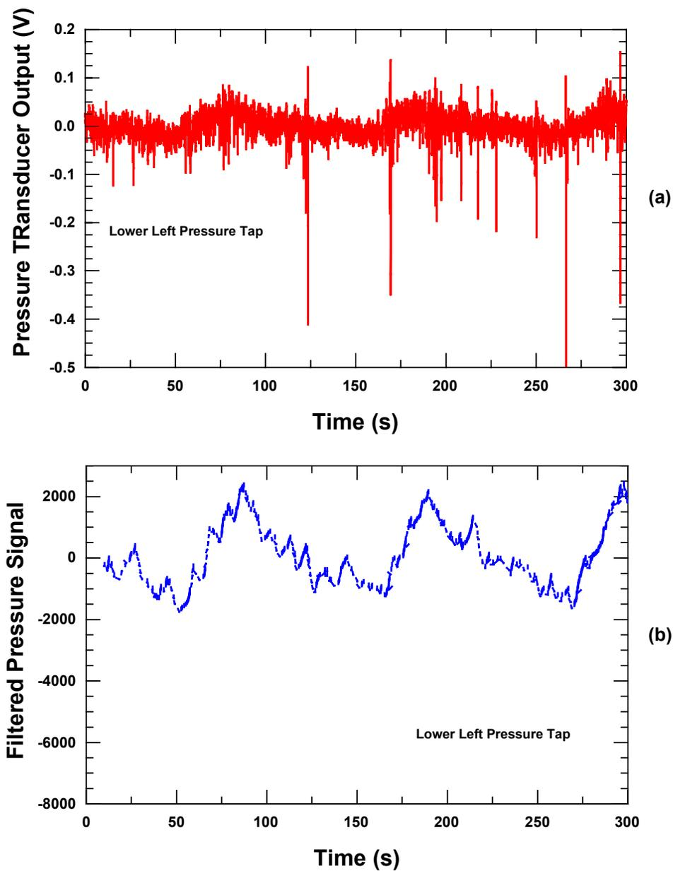
**Figure 7.** (a) Original time series from the bottom left pressure tap during an episode where the bubble plume was shifted to the right. Fluidizing air flow is 1.56 times the minimum. (b) Bottom left pressure signal after low-pass filtering with zero-phase-shift filter.
