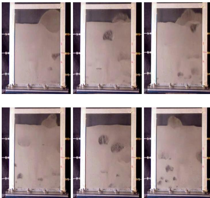
Figure 2. Example video images (randomly selected) from the 2-D bed illustrating bubble concentration toward the right side (top row) and even bubble distribution (bottom row). Fluidizing air flow is 2.08 times the minimum.
