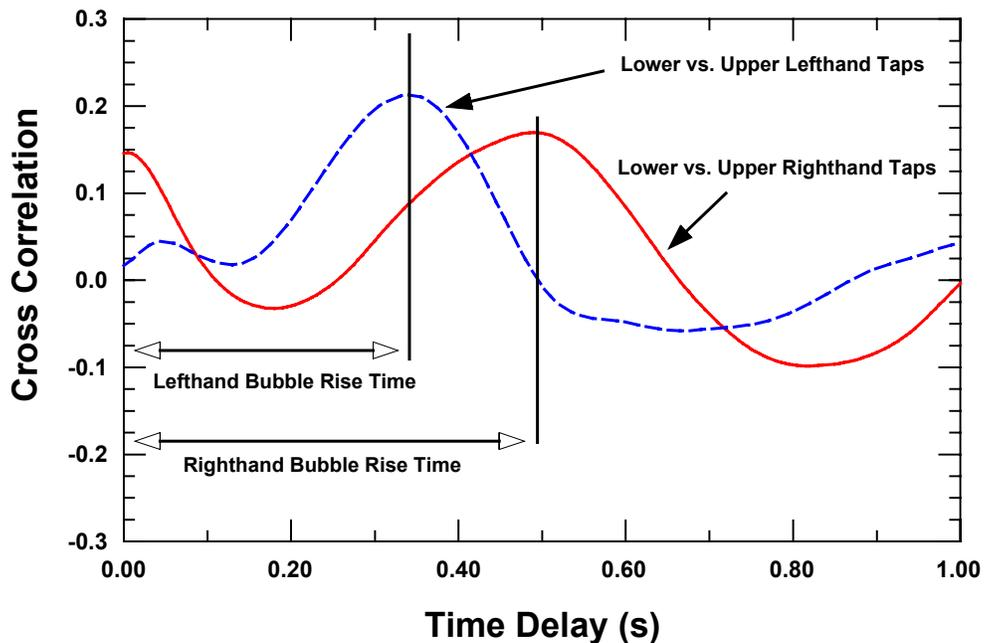
**Figure 5.** Cross correlation between vertically spaced pressure taps. Bubble plume is shifted to the left. Fluidizing air flow is 2.35 times the minimum.
