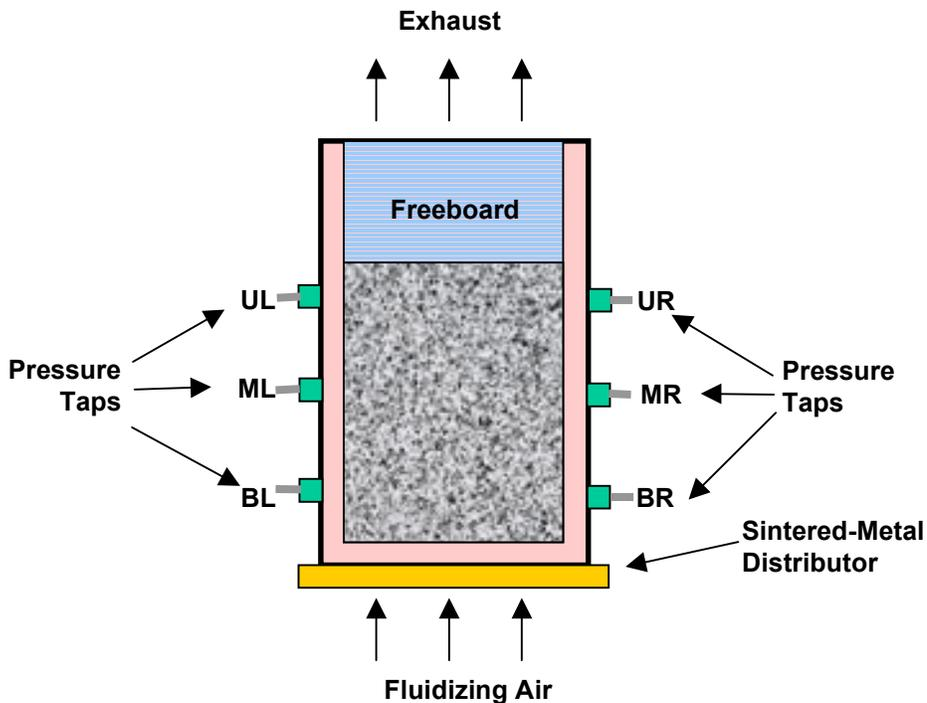
Figure 1. Schematic of two-dimensional fluidized bed.
