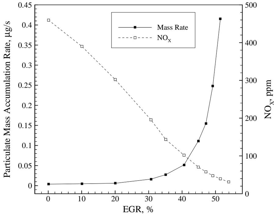
represents a region where the engine out particulate mass and NO<sub>x</sub> concentration are minimized for this engine condition.
