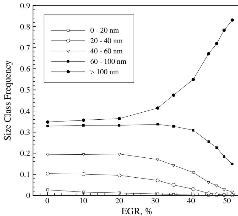
60-100 nm increases significantly at 30% EGR and continues to increase. The figure does appear to show that the smallest particles are contributing to the growth of the largest ones. The increase in larger particles is less steep than the increase in particle mass in Figure 4. The particle mass, however, increases as a function of the cube of particle diameter, and thus can be expected to increase more rapidly.
