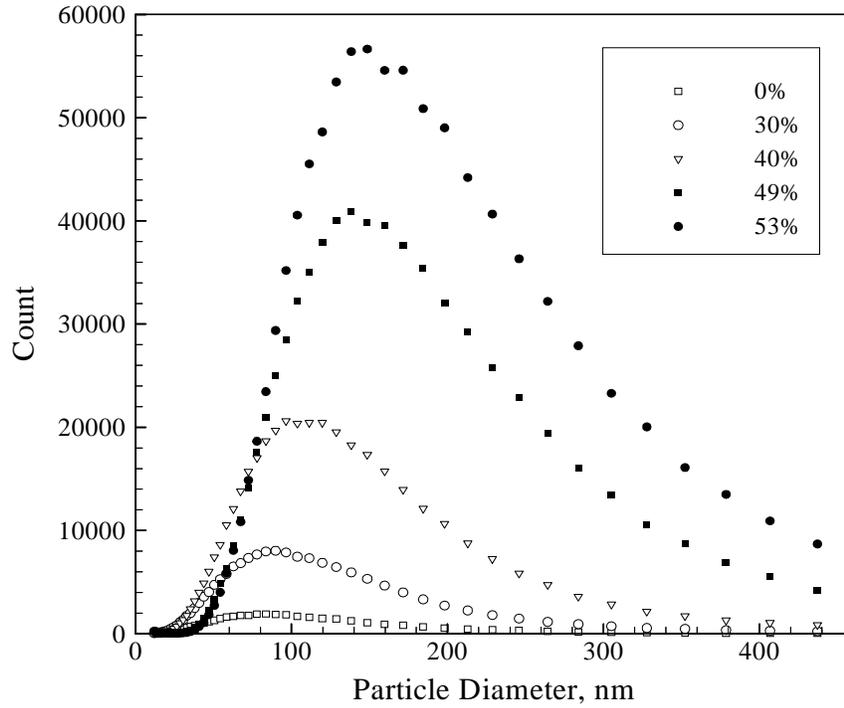
**Figure 6.** Frequency of occurrence of particle size classes as a function of EGR. Frequency of smaller particles decreases as the frequency of larger particles increases at higher EGR levels.
