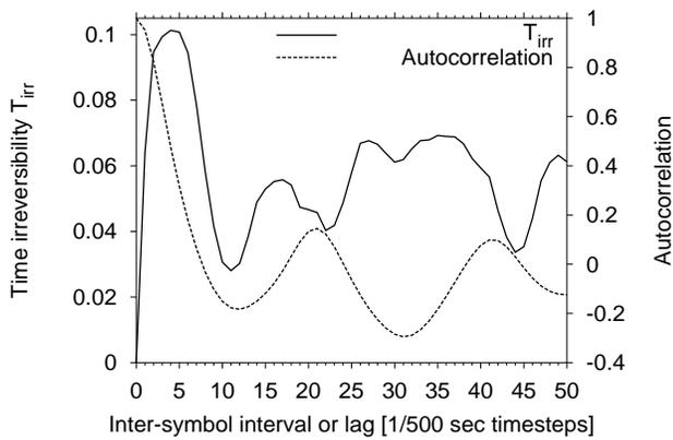
**Figure 11:** Time-irreversibility statistic as a function of inter-symbol interval and autocorrelation for  $Re_D = 291$ . Eight symbols of sequence length 2 were used to calculate differences between forward-time and reverse-time symbol-sequence histograms.
