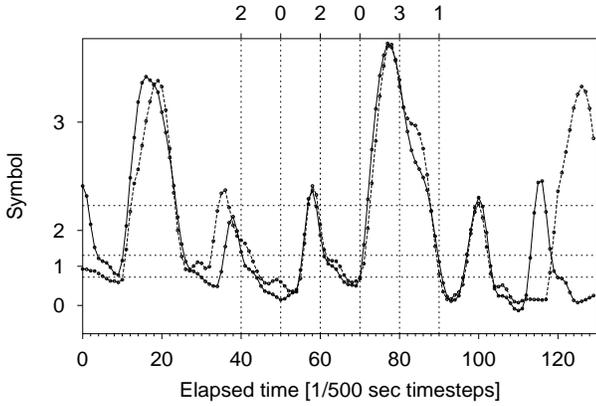
**Figure 9:** Repeating trajectory segments for set 1,  $Re_D = 291$ . Four symbols of sequence length 6 and inter-symbol interval of 0.02 sec were used to find sequence 202031 in both segments. The second segment (dashed line) occurred 5.9 sec after the first segment.
