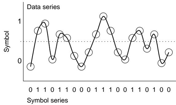
**Figure 2:** Illustration of symbolization. Each value in the symbol series at the bottom corresponds to the point directly above in the data series.
