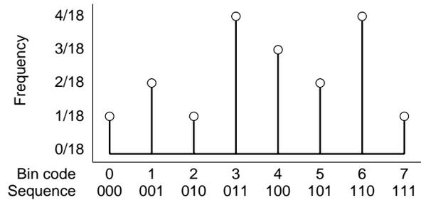
**Figure 3:** Example symbol-sequence histogram for the symbol series shown in Fig. 2. Note that sequences 011 and 110 are most frequent.
