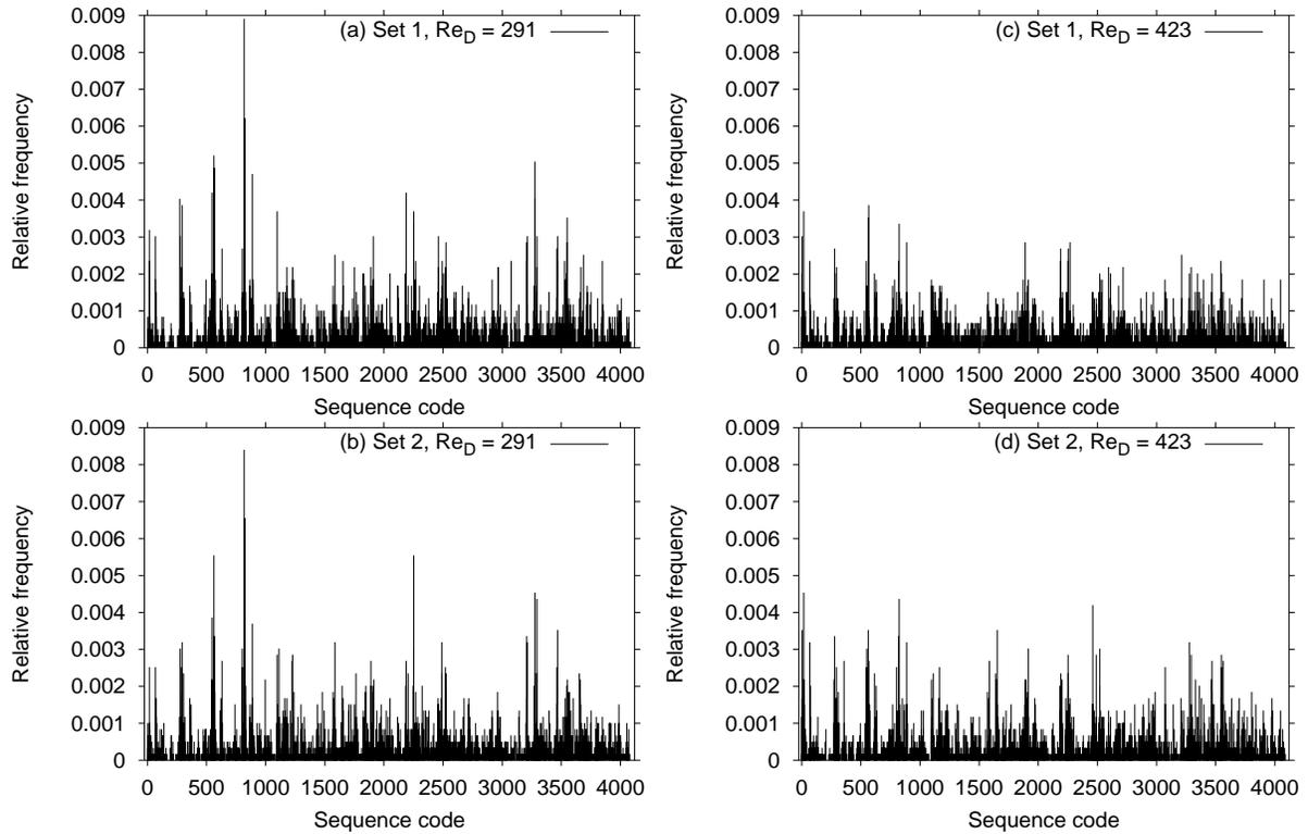
**Figure 7:** Symbol-sequence histograms for two replicate pairs (repeat experiments at the same flow conditions). Four symbols of sequence length 6 and inter-symbol interval of 0.02 sec were used.
