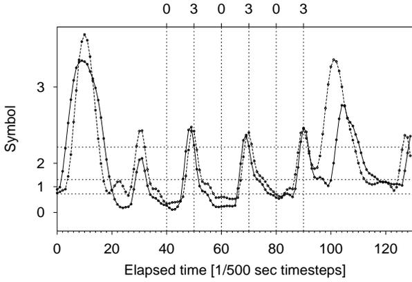
**Figure 8:** Repeating trajectory segments for set 1,  $Re_D = 291$ . Four symbols of sequence length 6 and inter-symbol interval of 0.02 sec were used to find sequence 030303 in both segments. The second segment (dashed line) occurred 1.6 sec after the first segment.
