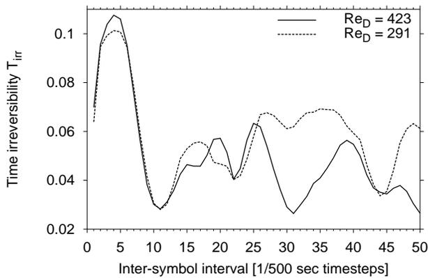
**Figure 12:** Time-irreversibility statistic as a function of inter-symbol interval for two of the data sets used in Fig. 1.
