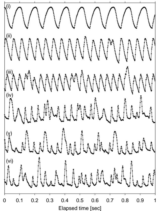
**Figure 5:** Example time series for the pressure transducer at six injector flows ( $Re_D$ ): (i) 13, (ii) 63, (iii) 100, (iv) 216, (v) 291 and (vi) 423.
