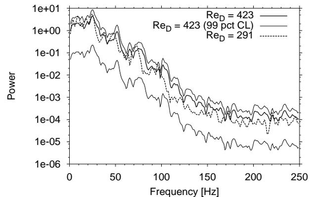
**Figure 1:** Fourier power spectra for two injection-rate conditions. Upper and lower curves indicate 99% confidence limits.
